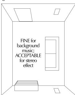
Russound In-wall speakers may be used for rear surround sound channels by placing them (1) behind, (2) on each side of the viewing position or (3) in the ceiling just behind the viewers. The SP550.2 & SP650.1 speakers also make excellent, unobtrusive front channel home theater speakers for 5 channel listening.
